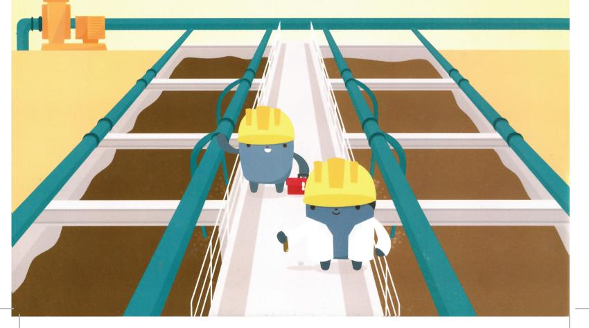
Grease and oils float to the top and are removed while sludge settles on the bottom.
