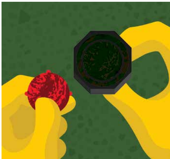
2.5 Remove the top rubber disc from inside of the bottom fitting. Blockages here prevent water draining through the small hole after every rainfall event.
