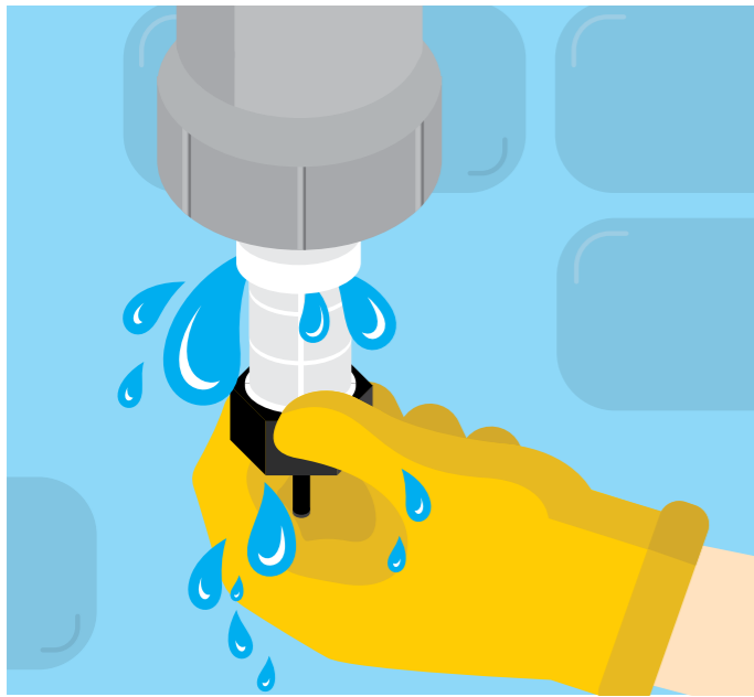
2.3. Remove the filter taking care to avoid being splashed by dirty water as it rushes out.
