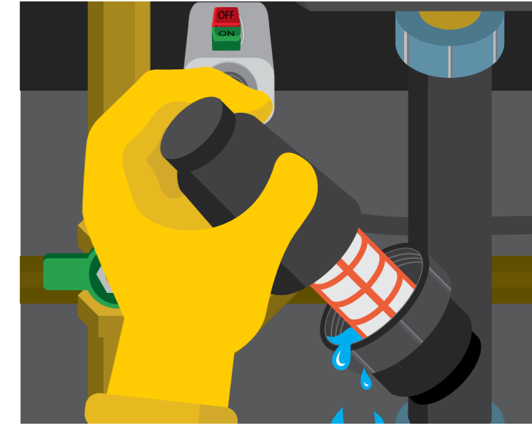
7.6 Slowly unscrew the body of the cartridge filter to release pressure and excess water.
