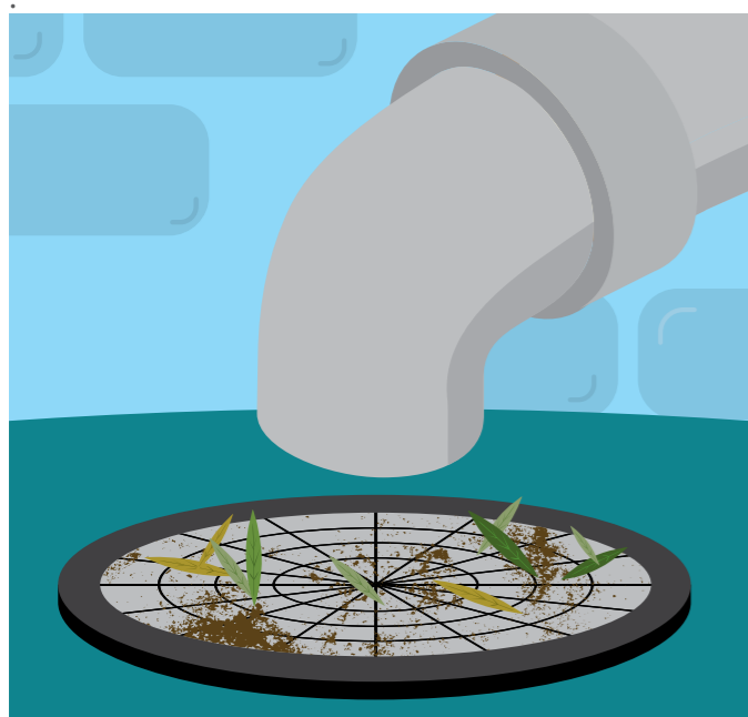
3.1 Locate your inlet screen. This is often found screwed into the hole below the inlet pipe at the top of the tank
