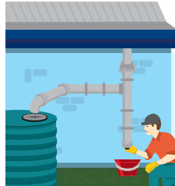
2.1 Locate your first flush device and place a bucket underneath.
