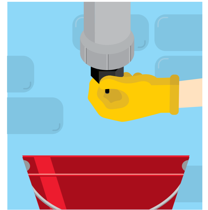
2.2 Unscrew the small bottom fitting slowly. If you have an irrigation hose attached, remove this from the bottom fitting.
