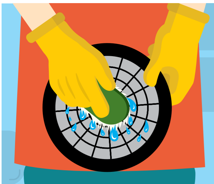
3.1 Locate your inlet screen. This is often found screwed into the hole below the inlet pipe at the top of the tank
