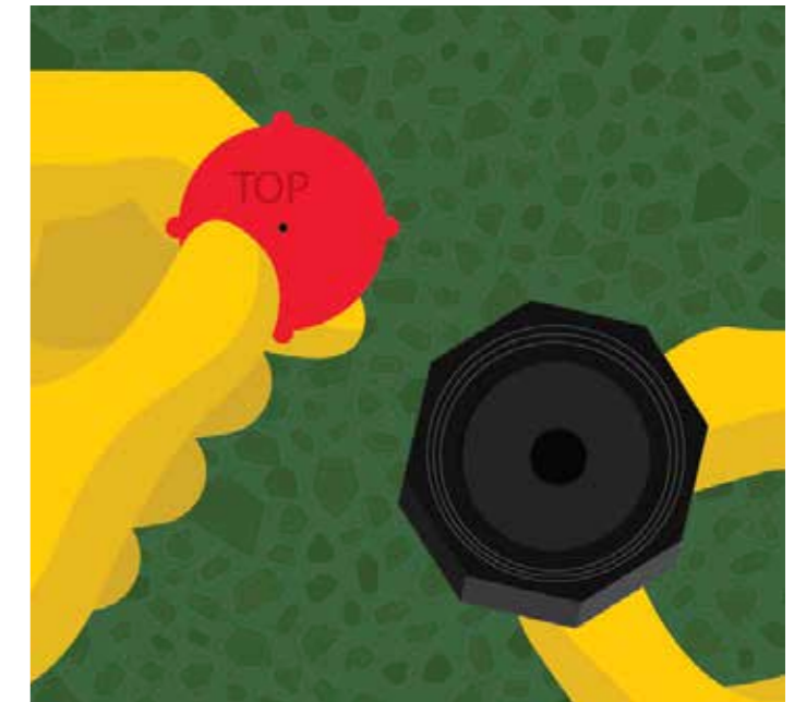
2.8 Check that the rubber disc is clean and not damaged. Replace if necessary.
