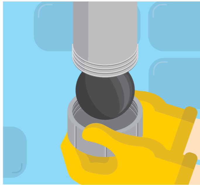
2.4 Unscrew the larger bottom cap containing the floater ball and debris caught by the first flush chamber.
