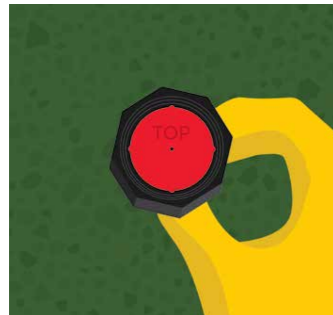
2.9 Place the rubber disc back inside the bottom fitting and ensure the word 'TOP' is visible. Reassemble filter and small bottom fitting to your first flush device.
