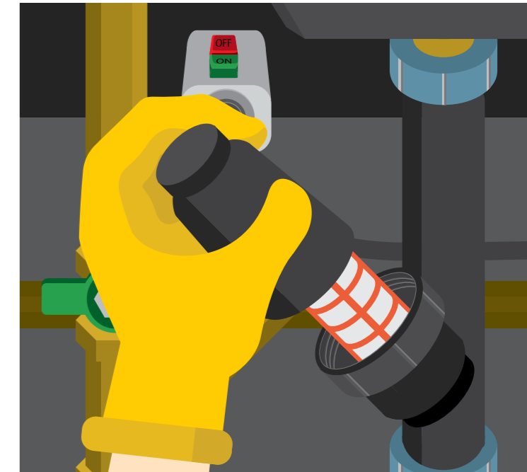
7.8 Reassemble back together and ensure the switch to mains water and pumps are turned back on.
